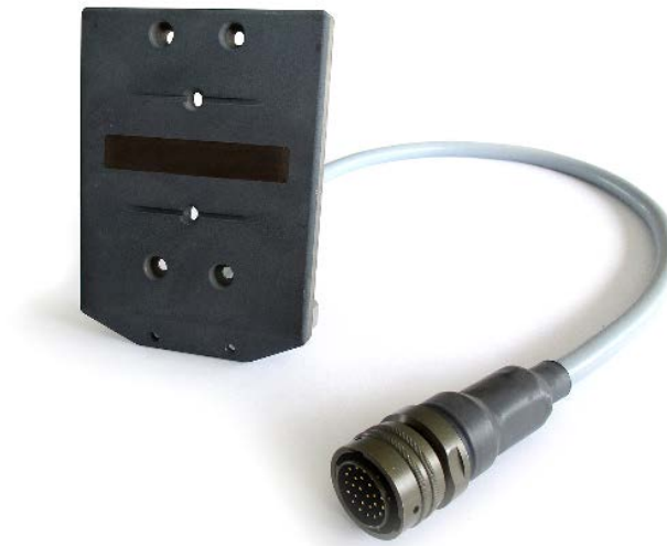
Fig. 2 – Multichannel Electromagnetic-acoustic Transducer
